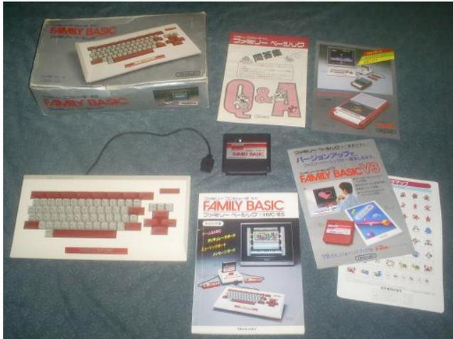
**Figure 2: Family BASIC keyboard, cartridge, and cassette data recorder connect to the Famicom System**
